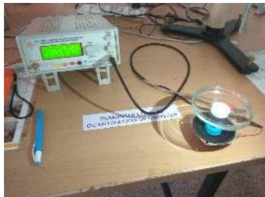
Fig. 1 Shows a signal generator sinusoidal (1-100 Hz)
